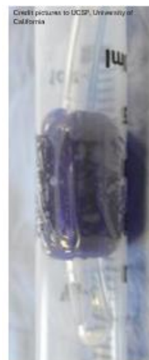
Benchtop study showing fluid travelling passed ETT cuff involutions
