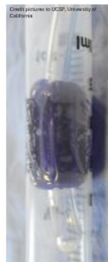
Benchtop study showing fluid travelling past ETT cuff involutions
